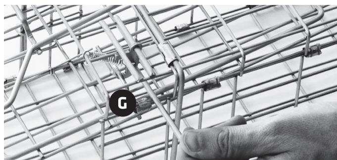
6. Now press on the clamping bracket to be able to fold the front door upwards. It automatically engages in the door holding hook.
